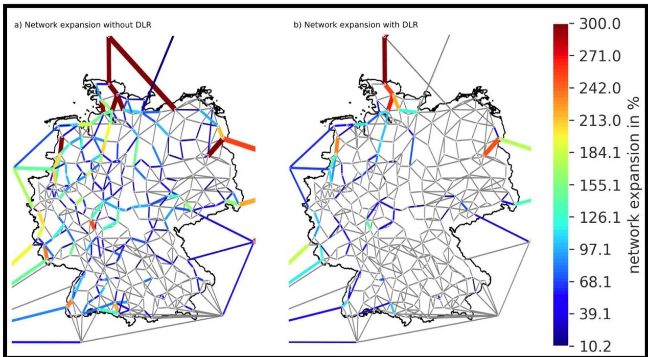
Figure 6-1: Required network expansion in absolute values for scenario eGo 100. a) without DLR. b) with DLR.
