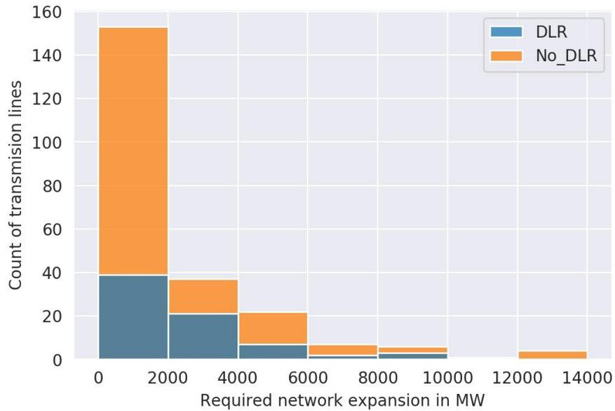
Figure 6-3: Histogram network expansion requirements with and without DLR. Source: author
