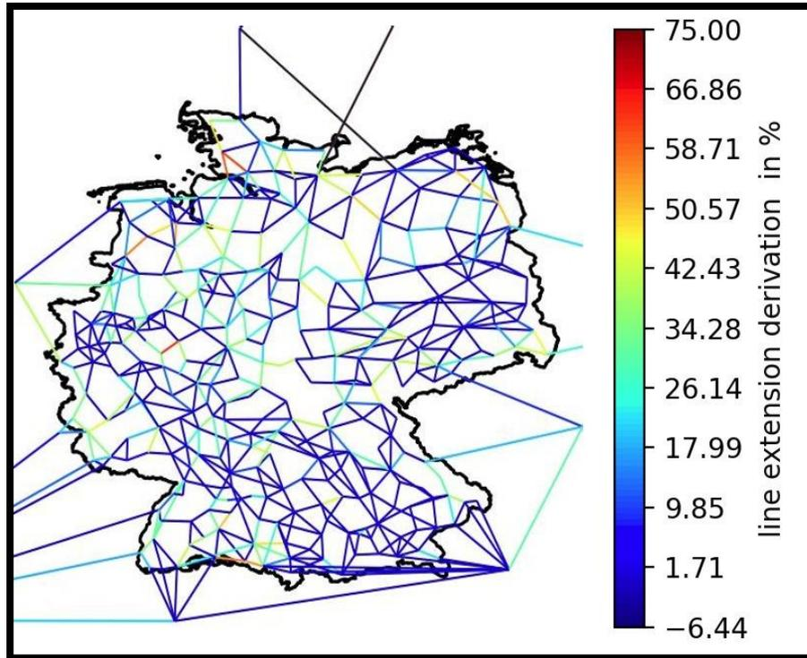
Figure 6-2: Network expansion difference between the scenarios with and without DLR. Source: author
