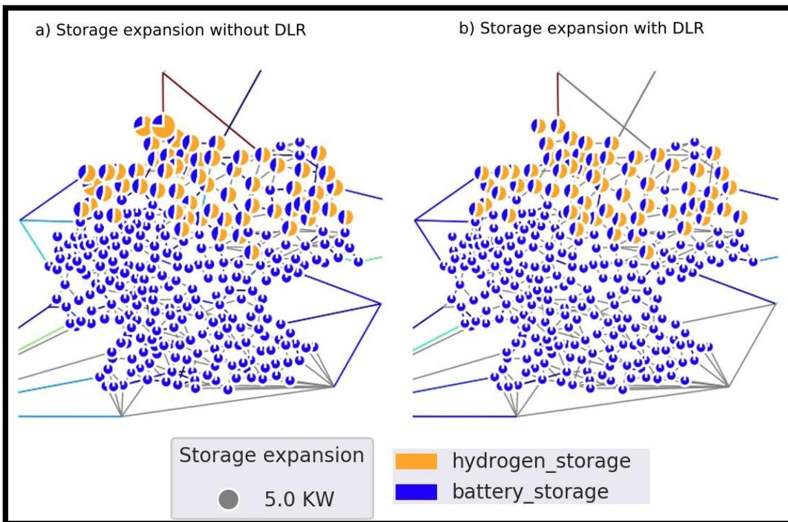
Figure 6-8: Require storage expansion for scenario eGo 100. a) Without DLR. b) With DLR. Source: author
