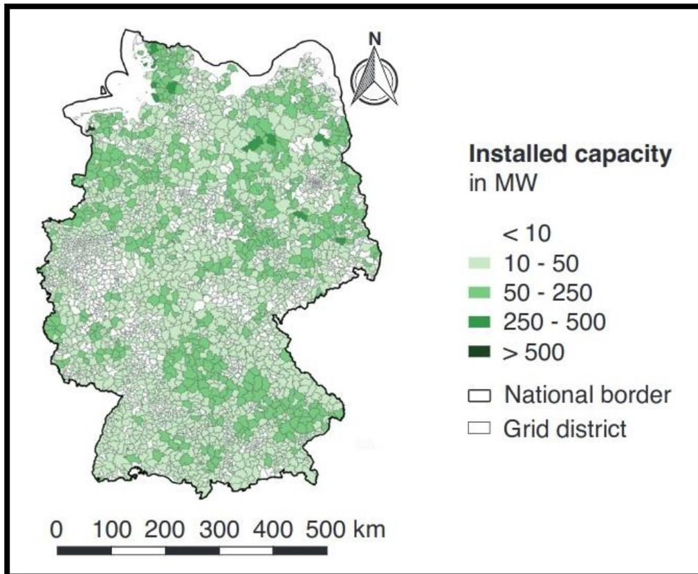
Figure 5-2: installed capacity for the scenario eGo 100. Source: Hülk et al., 2017
